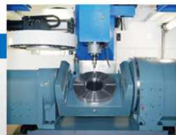
ERT500 The integrated design takes out the table and can bear more weight than conventional add-on five axis table. There are less interference in the large part machining by this design.
