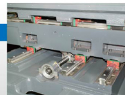
There are three linear ways that can bear the heavy weight from the load or five axis table but still keep good accuracy.
