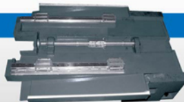
The rigid box type base let the Y axis travel up to 650 mm and keeps better accuracy among similar models.
