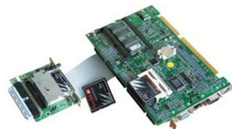
Compact Flash Memory Card Optional Compact Flash Memory Card provides a multi access environment
